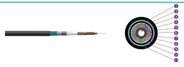
1,Fibre 2,Loose Tube 3,Tube Filling Compound 4,Strength Member 5,PE Layer 6,Cable Filling Compound 7,APL 8,LSZH Inner Sheath 9,Cable Filling Compound 10,PSP 11,LSZH Outer Sheath
