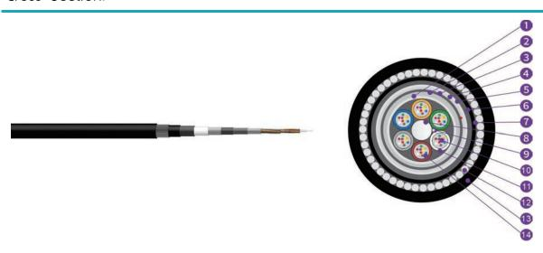
1,Water Blocking Tape 2,Fire Resistance Tape 3,LSZH Inner Sheath 4,Water Blocking Tape 5,APL 6,HDPE Second Sheath 7,PA Sheath 8,Strength Member 9,Water Blocking Yarn 10,Fibre 11,Loose Tube 12,Steel Wire 13,LSZH Outer Sheath 14,Tube Filling Compound
