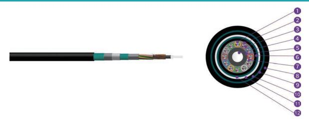
1,Fibre 2,Loose Tube 3,Tube Filling Compound 4,Strength Member 5,PE Layer 6,Fire Resistance Tape 7,Water Blocking Yarn 8,LSZH Outer Sheath 9,PSP 10,Fire Resistance Tape 11,LSZH Inner Sheath 12,PSP
