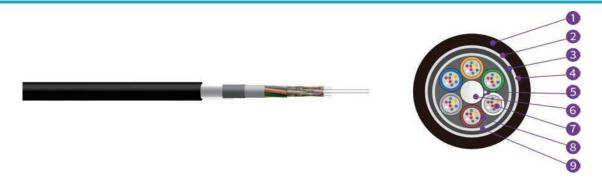
1,LSZH Sheath 2,Glass Fibre Yarn 3,Fire Resistance Tape 4,Ripcord 5,Water Blocking Yarn 6,Strength Member 7,Fibre 8,Loose Tube 9,Water Blocking Tape
