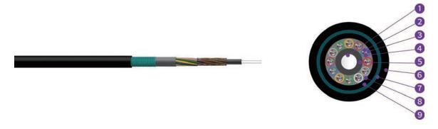
1,Strength Member 2,Fibre 3,Loose Tube 4,Tube Filling Compound 5,PE Layer 6,LSZH Sheath 7,PSP 8,Water Blocking Yarn 9,Fire Resistance Tape
