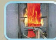
Fire Propagation Test On Bunched Cables (IEC 60332-3)
