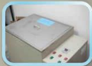
Thermostatic Water Tank
