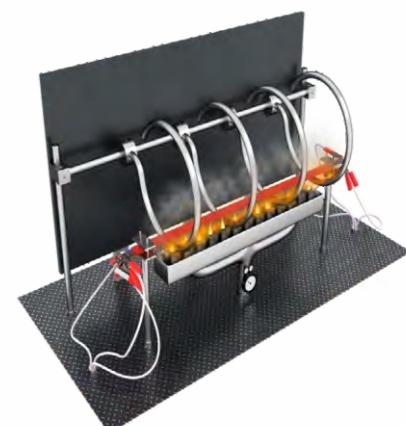
This test is carried out to verify circuit integrity even during a fire. A sample of cable is held on a flame at about 750°C for a period of minimum 90 min, under rated voltage.
