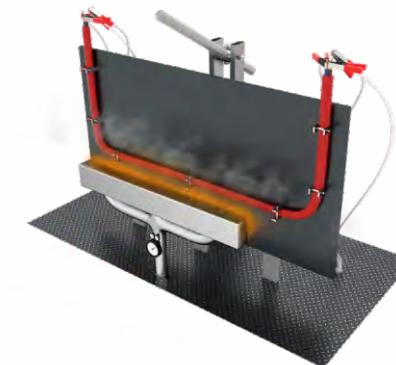
This test is carried out to verify the circuit integrity of cables exposed to fire at 830°C and mechanical shocks.
