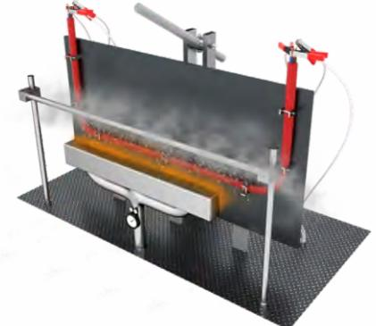
This test is carried out to verify circuit integrity during a fire. The cable is exposed to a flame at 930°C and mechanical shocks for 60 minutes and additional 60 minutes to flame, mechanical shocks and water spray.
