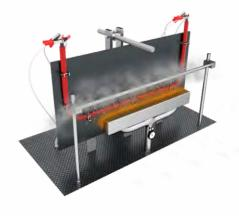
This test is carried out to verify circuit integrity during a fire.
