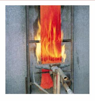
Samples of cables 3,5 m long in quantities required by standard are installed on a ladder inside a metallic cabinet. They are subjected to the action of a flame at 750°C for a specific time (20 or 40 minutes).
