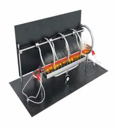
This test is carried out to verify circuit integrity even during a fire. A sample of cable is held on a flame at about 750°C for a period of minimum 90 min, under rated voltage.
