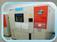
Climatic Test Chamber
